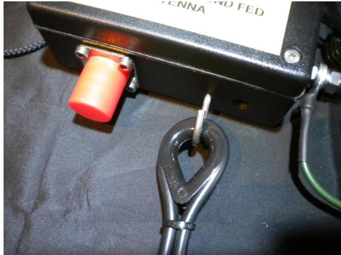
Finally, unwind the green Kevlar wire from the winding spool and slope it down the garden, tie it off to a fence, post or tree with the supplied cord that is on the winding spool, try to keep the end of the green Kevlar wire a couple of metres above ground.
